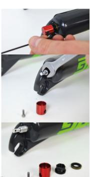
4. Frog 69/72 MTB Only. Remove Rebound control knob using 2mm Allen key. Then use a 10mm spanner to remove the nut and spacer.
