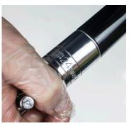
12. Re-tighten in the inner stanchions. 18Nm
