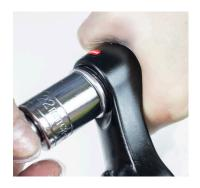
8. Tighten using 22mm socket. 18Nm
