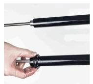
17. Slide NEW wiper seals & soaked foam rings onto the Inner Stanchion legs and lightly grease.
