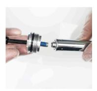
1. Attach alloy lockout top cap to oil cartridge using the lockout assembly bolt.
