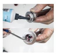
2. Add a small amount of grease to each of the 3 holes in the lockout assembly bolt.
