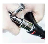
11. Unscrew alloy lockout top cap using either a 22mm or 24mm socket depending on version.
