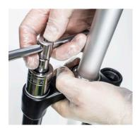
15. Re-fit the Alloy Air valve seal top cap using 24mm socket. 18Nm
