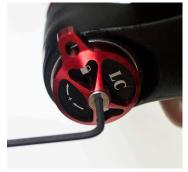
24. Re-fit red lockout adjustment lever. The fork should be in locked out position with cap in the appropriate position.
