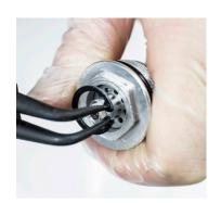
5. Re-fit circlip, locating correctly into the recess.
