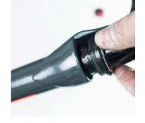
26. Finally, re-fit the blue air valve dust cap. Test fork the correct way up on a soft surface. Re-fit forks to frame.
