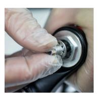
7. Lift out lockout control rod.
