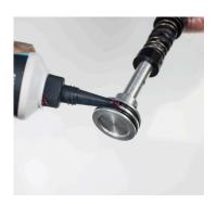
9. Grease air valve piston assembly.
