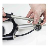
25. Pressurise the fork using a shock pump to approx. 50psi. (0271)
