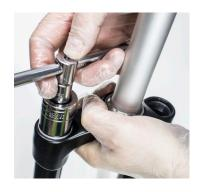
16. Unscrew alloy air valve seal top cap using 24mm socket.
