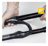
20. Slide the inner and outer stanchions back together. **N.B. The fork brace is on the**
