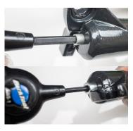
9. Undo lower stanchion bottom bolts. 6mm/5mm. N.B Compress forks & make an initial sharp twist to break thread seal.
