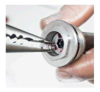
3. Carefully relocate the springs and ball bearings.
