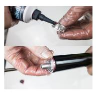
11. Grease the thread on the Bottom Alloy air cap
