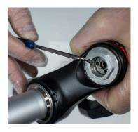
8. Remove 3 Ball bearings and springs using a magnetic pick.
