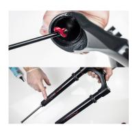
19. Grease the outer stanchion bushings and foam rings using a dowel rod.
