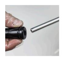
14. Remove rubber top out buffer from inner air rod.
