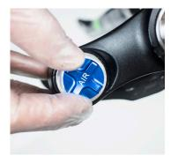
2. Remove blue air valve dust cap.
