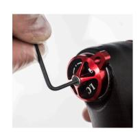
5. Remove red lockout adjustment lever with either a 2.5mm hex or screwdriver depending on version.
