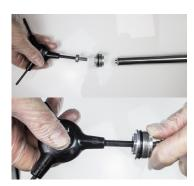
13. Holding the oil cartridge firmly undo the top bolt inside the alloy top cat.
