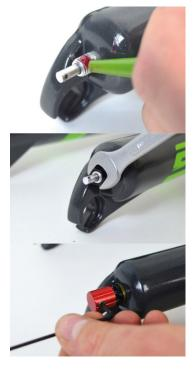
23. Re-assemble rebound control knob. Apply a small amount of grease to the rebound thread. Reinstall the spacer and nut with a 10mm spanner. Install the switch with a 2mm allen key.
