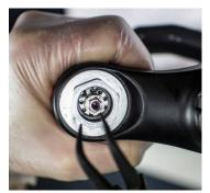
6. Remove circlip.
