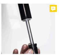
13. Pull out Inner air rod and fit rubber top out buffer. Then slide the inner and outer stanchions back together.
