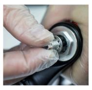
4. Relocate the lockout control rod.N.B take care not to dislodge the ball bearings.
