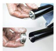
15. Slide inner air rod up and use a 24mm socket to undo and remove alloy bottom air cap. Then slide out air valve piston assembly.
